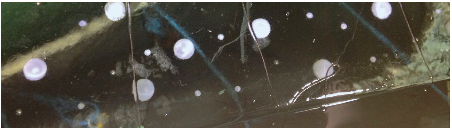
Figure 3. Target spheres were frozen in bubble-free ice blocks in an attempt to identify solid and hollow inclusions in ice using an echosounder.
