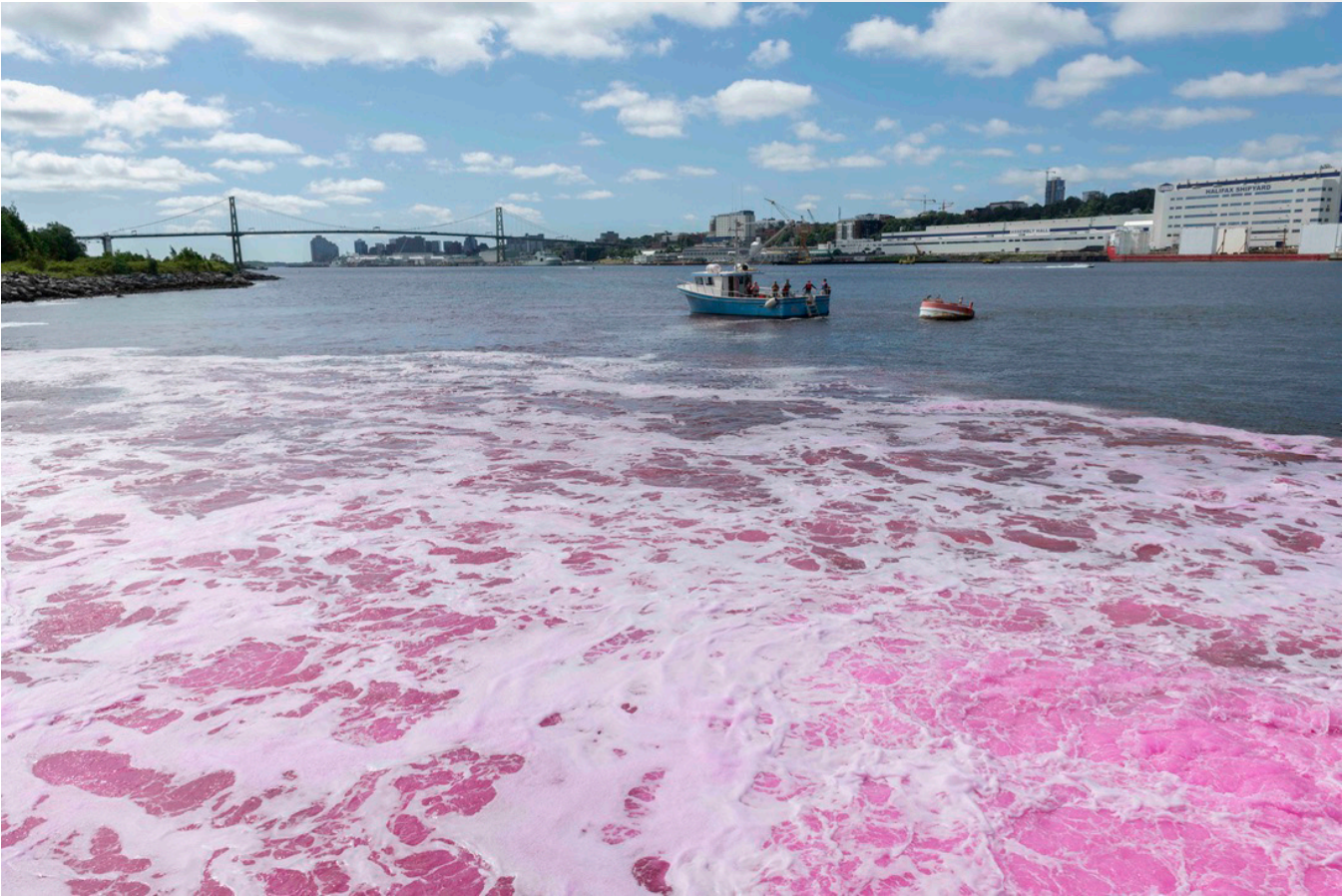
▲ The crew aboard the Eastcom observes the edge of the Rhodamine plume during a dye release experiment. Image credit: Dalhousie University
